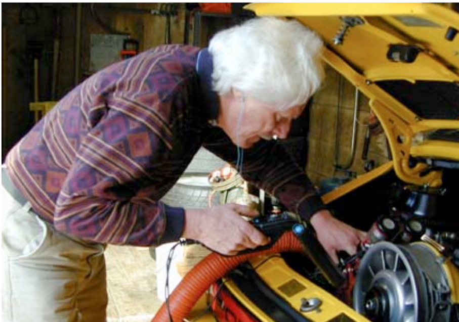
Timing the engine at 6,000 rpm requires racer earplugs. The noise is unbearable.
