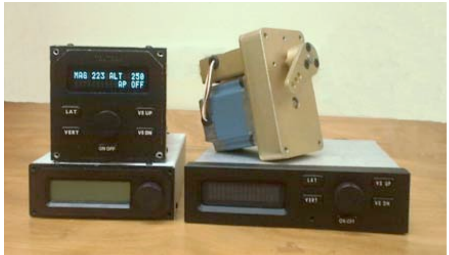
TrueTrak autopilots start with a simple, all-electric, single-axis autopilot and offer options up to full-featured three-axis autopilots.
