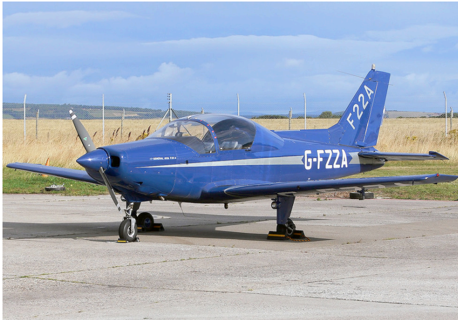
General Avia F.22B with 160-hp engine, fixed gear and fixed-pitch propeller.
