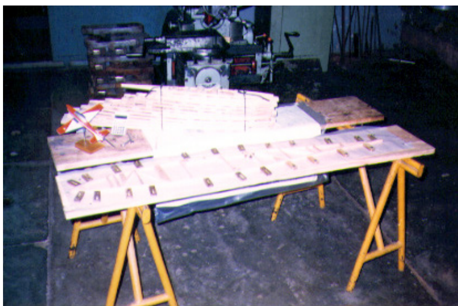
Top and center: Marcello Bellodi's tail surface assembly jig. Bottom: Marcello Bellodi's wing rib jig is adjustable and is used to make all of the wing ribs.
