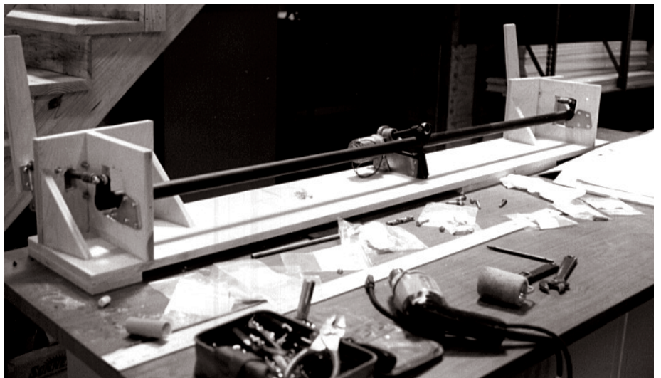
Top: The first of the fuselage frame laminations.
