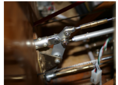
Pitch pushrod and servo
