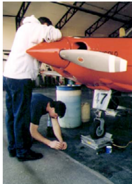
Above: Hanging a plumb line to locate the datum.
