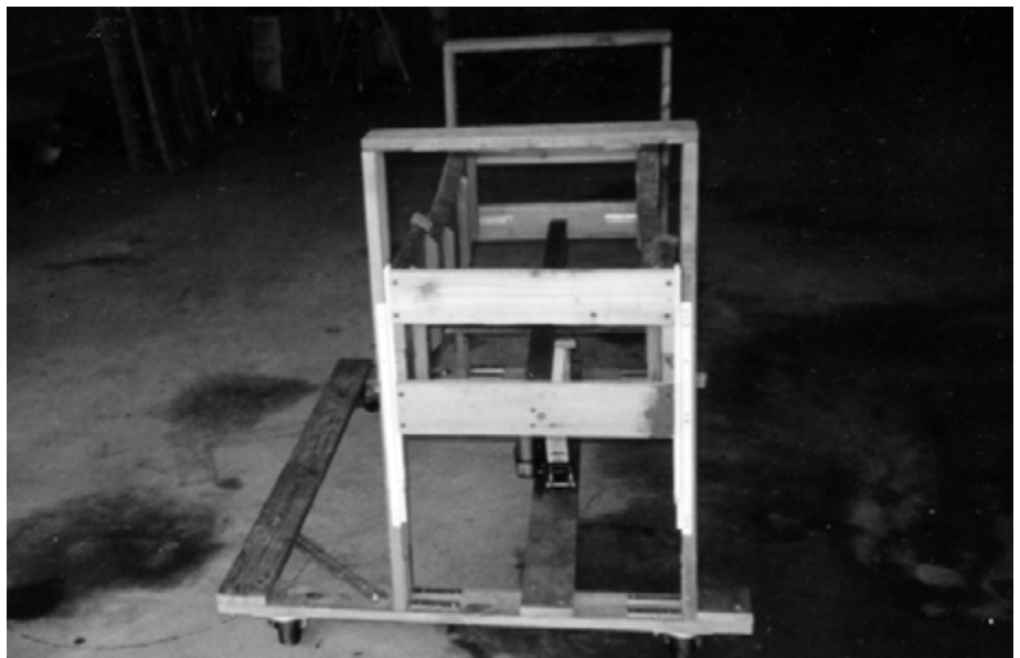
Cecil Rives got tired of looking for someone to help him every time he wanted to take the cowling off, so he came up with this gizmo.
