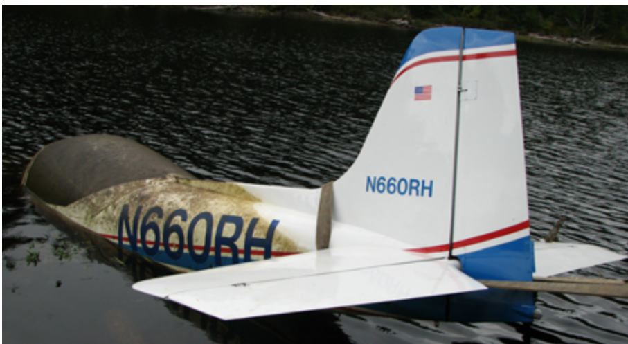
Pulling the Falco to shore. Note the tree top section in the right horizontal stabilizer.
