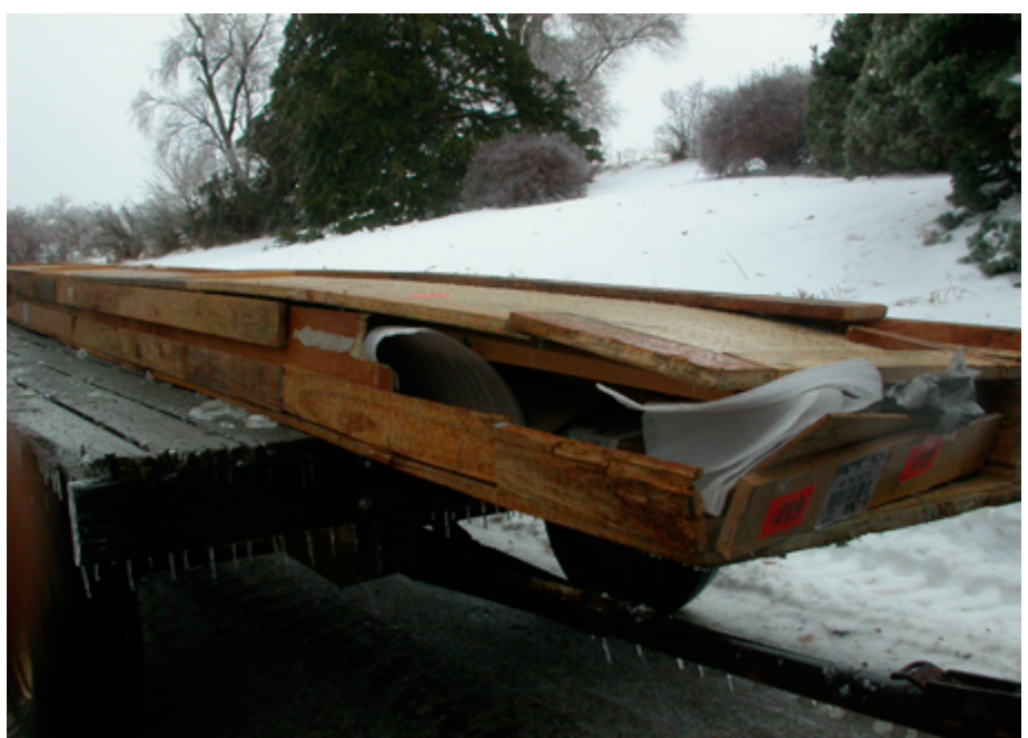
Shawn and Susan crating main wing spar kit for Jerry Mulliken. All spar crates get the 'Great Bird of Falco' on them. Then look at what the trucking company did with this! They ran a fork-lift into it, but luckily there was no damage beyond the crate.
