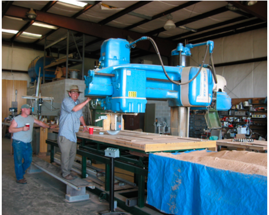
Walter with his radial arm saw made from a radial drill. Bill Keller to the left.
