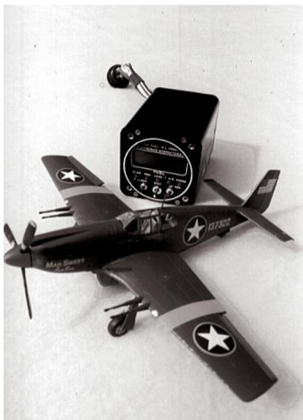
tems complain of instrument inaccuracy ranging all the way up to 10-percent errors in fuel actually burned versus fuel-used figures computed by the Shadin.
