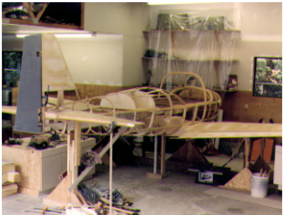
Dave Nason's Falco takes shape in Kent, Washington. This was the state of the airplane as of early September, with the wing and tail 'glassed and ready for paint.
