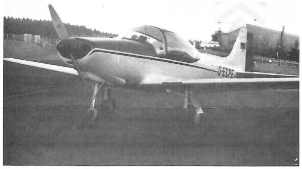
Lutz Gosser sent us the above photo of his Falco. The airframe has been completely redone and Mr. Gosser is now adding a new engine, a constant speed propeller, new wheels and a new brake system. His Falco is painted in a lovely scheme being white with orange-red spinner, rudder and wing tips, and dark blue trim elsewhere. The carburetor intake appears to have been modified -- either covered over or with a screen in the front.
